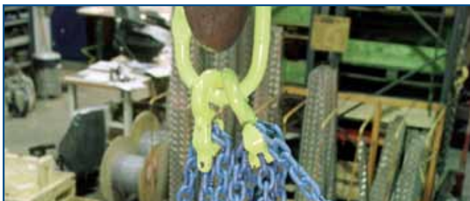
Fig. 7. "A three-leg, fully adjustable sling."
